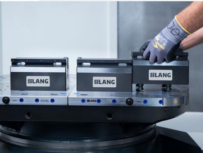
Adding further bases for an increased clamping range
