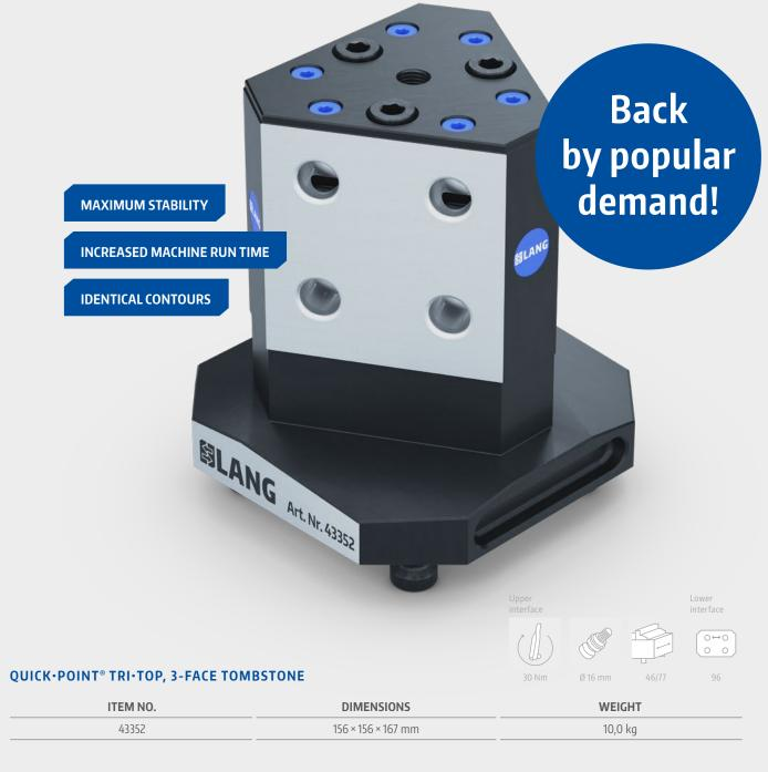
The Tri-Top returns in a fresh design! With its **sturdy steel base body**, the 3-face tombstone is a guarantee for maximum precision. Despite its robustness, the Tri-Top remains handy and has the same interference contours as its predecessor. The 3-fold zero point mounting, suitable for Makro·Grip® 46 and 77, **reduces downtimes and tool changes** in milling operations.
