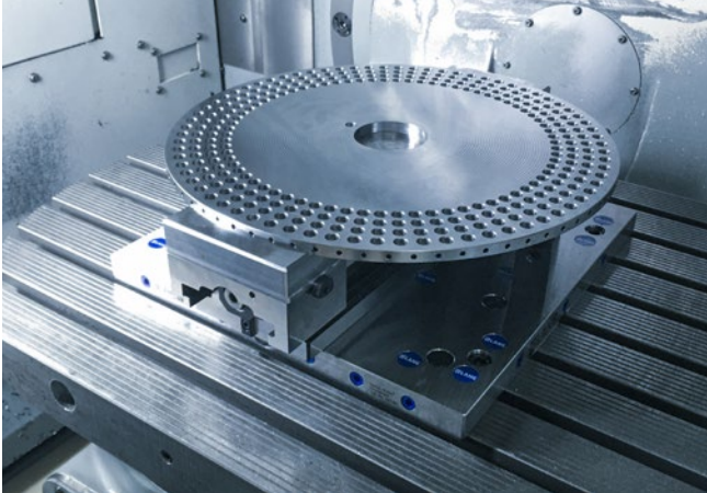
Part size: Ø 420 x 10 mm, material: 1.7131, Makro-Grip® Ultra Basic Set 410 S with Avanti top jaws
