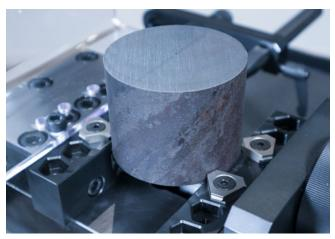
The external pre-stamping process of the blank ensures the form-closure effect between stamping indentation and serration of the clamping jaw.
