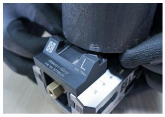
The clamping jaws grip the pre-stamped workpiece in four indentations.
